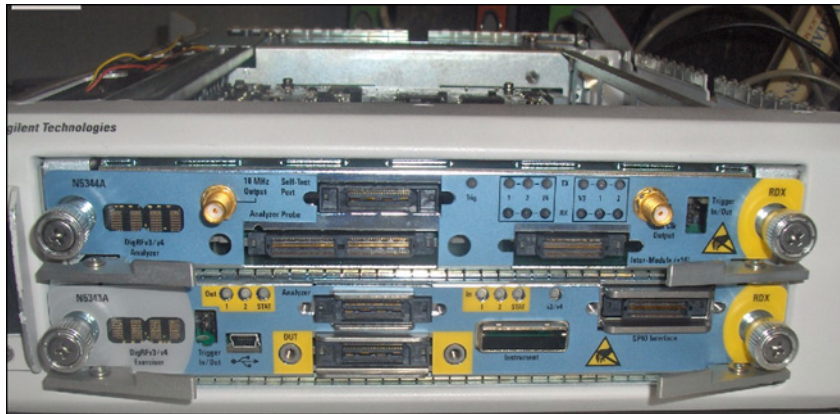
Figure 1 Modules in N5302A chassis
